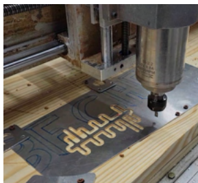
CNC routing the antenna reflectors and deflectors I designed
