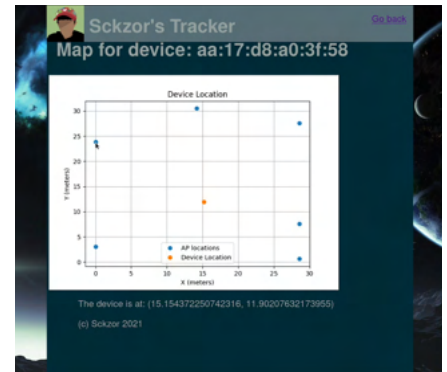
A map generated by my system showing the location of a mobile device
